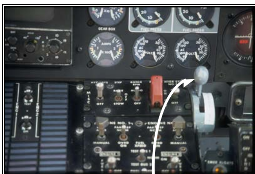
Figure 3-24 Defrost Control Lever
