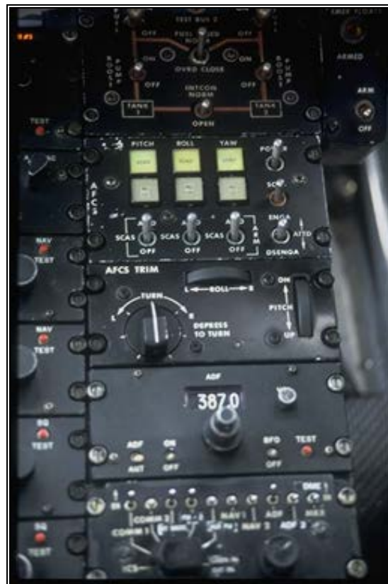
Figure 3-21 AFCS Control Panel (Bell)
