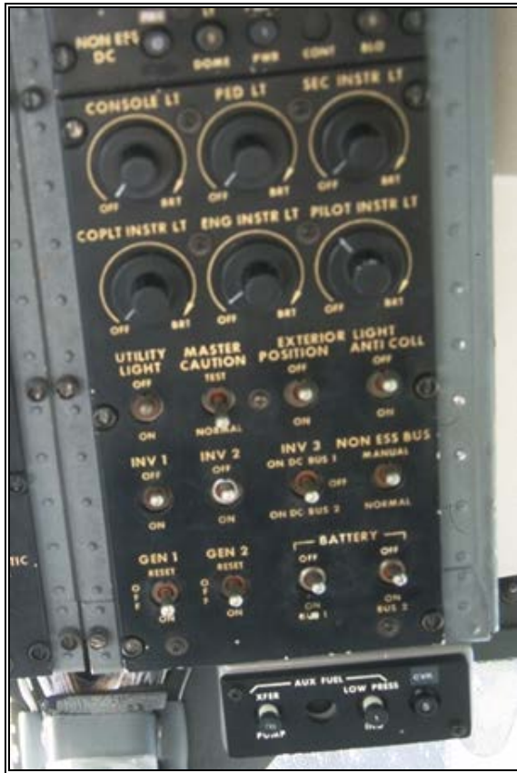
Figure 3-25 Forward Right Overhead Console
